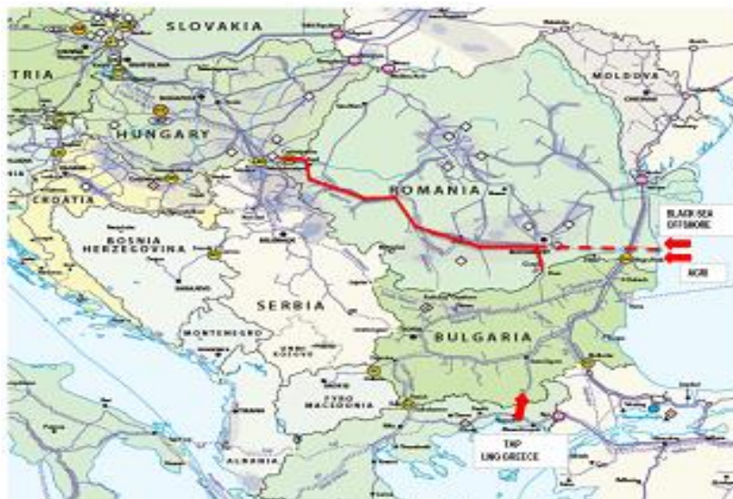
Figure 2 – The interconnection points of the Romanian gas transmission system with the similar Bulgarian and Hungarian systems
