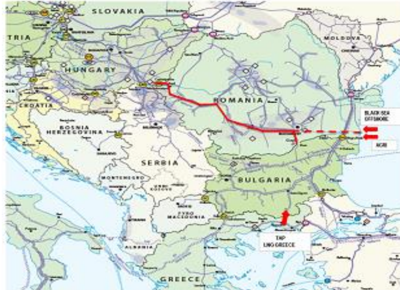
Figure 2 – The interconnection points of the Romanian gas transmission system with the similar Bulgarian and Hungarian systems
