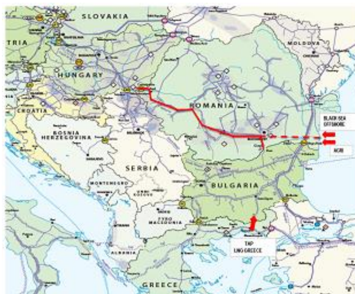
Figure 2– The interconnection points of the Romanian gas transmission system with the similar Bulgarian and Hungarian systems
