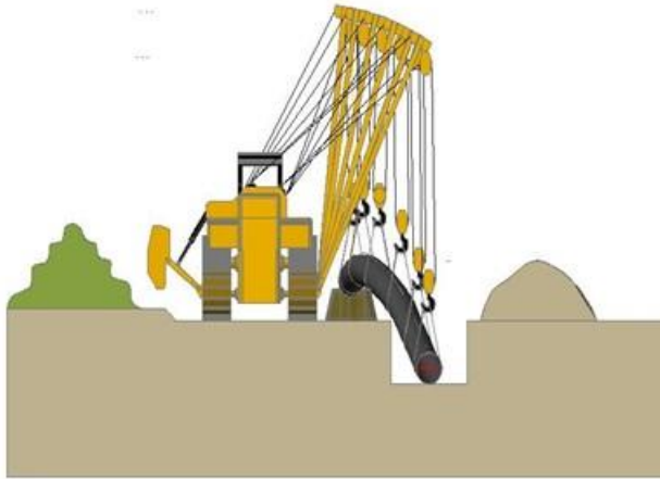
Figure 4.4 Schematic view of gas transmission pipeline laying
