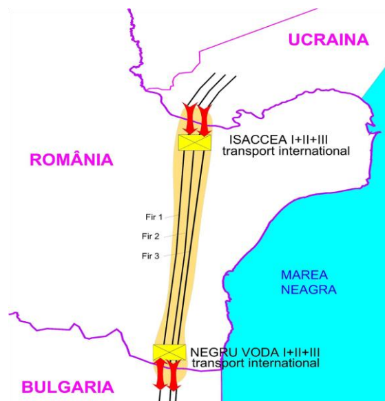
Fig. 12- International gas transmission pipelines
