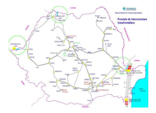
Apart from the abovementioned cross border interconnection points the Romanian transmission system also has 137 entry points from the production fields, 7 interface points with the undergoud storage facilities, 870 physical exit points to the distribution systems and 232 exit points to the consummers directly connected to the transmission system.
