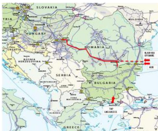
Fig. 10 - The interconnection points of the Romanian gas transmission system with the Bulgarian and Hungarian systems
